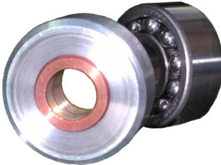
*Fig. 1.1. Homopolar induction bearing compared to a spherical ball bearing.*
