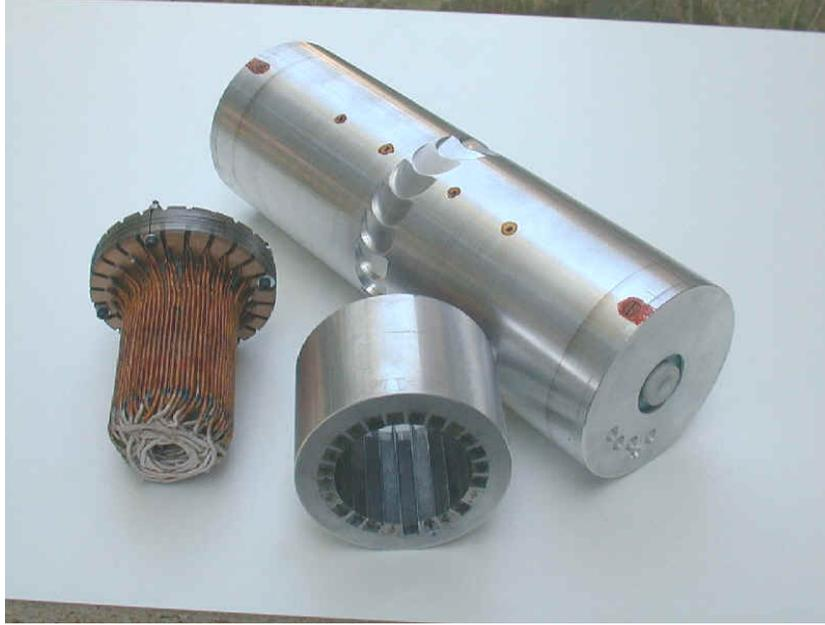
*Fig. 2.3. A prototype from Lausanne where Richard Post's bearing is evaluated.*
