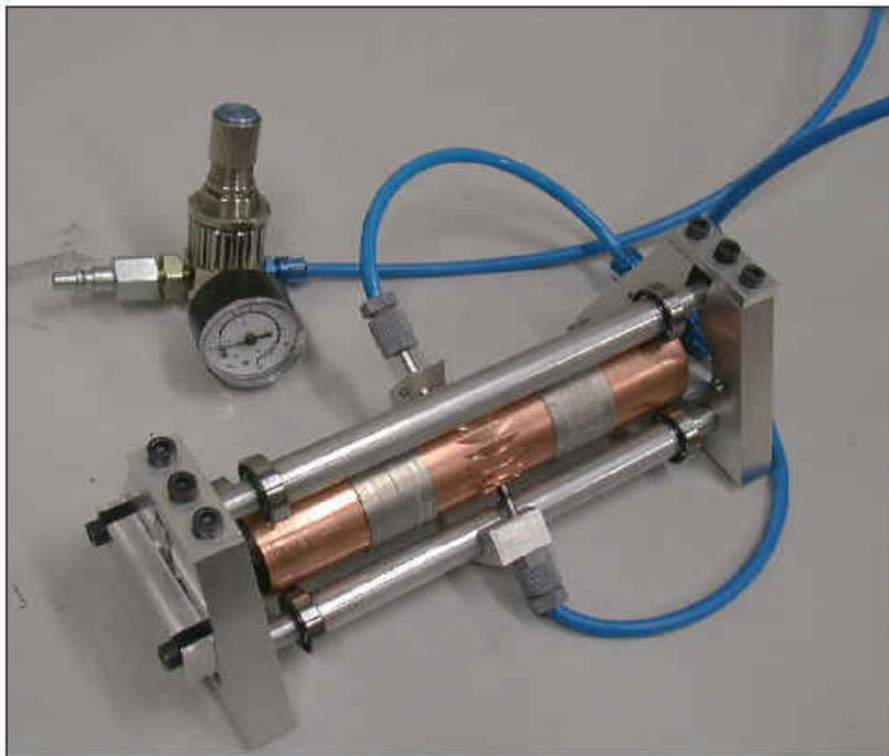
*Fig. 2.5. Swiss rotor with air turbine and homopolar bearings.*
